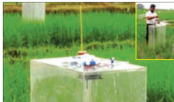
Closed chambers used for collection of air samples at regular intervals from the paddy fields
