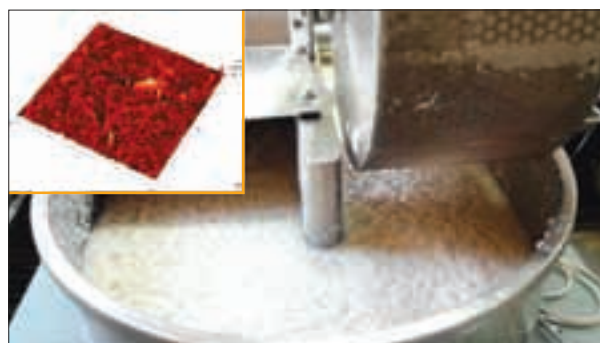
Nano-cellulose production process (inset: AFM image of nano-cellulose)
