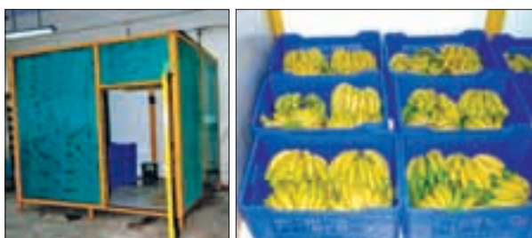
Collapsible ripening chamber for banana and other fruits
