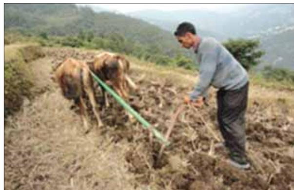
A wing- plough for shallow tillage and puddling up to 100-120- mm depth, weighing 8 kg, has a field capacity 0.025 ha/h for puddling and of 0.03 ha/h for tillage at speed of 2.2 and 2.4 km/h; ` 300/ha were saved by these implements compared to the traditional wooden- plough.
