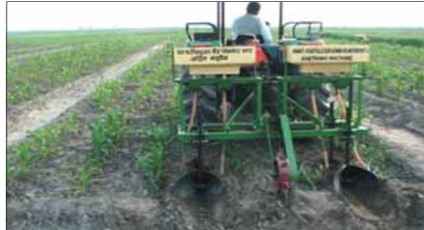
weeds in maize, sugarcane and potato having more than 0.50-m row-to-row spacing. The field capacity and efficiency of the machine are 0.56 ha/h and 82.4%, respectively, and with this, there is considerable saving in fertilizers, time and labour over the traditional method.
