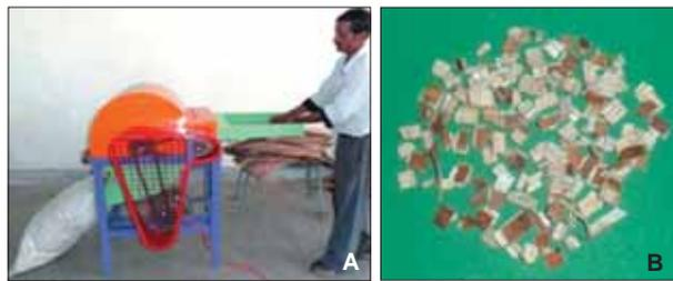
(A) Arecanut sheath shredder; (B) arecanut fodder
