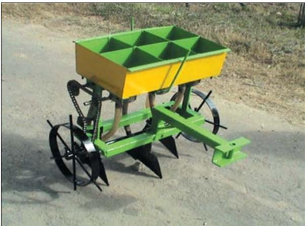
Power tiller-operated zero-till drill
