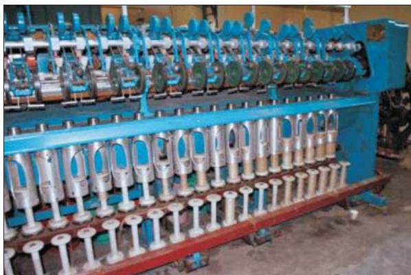
Automated flyer spinning machine for jute-coconut fibre
