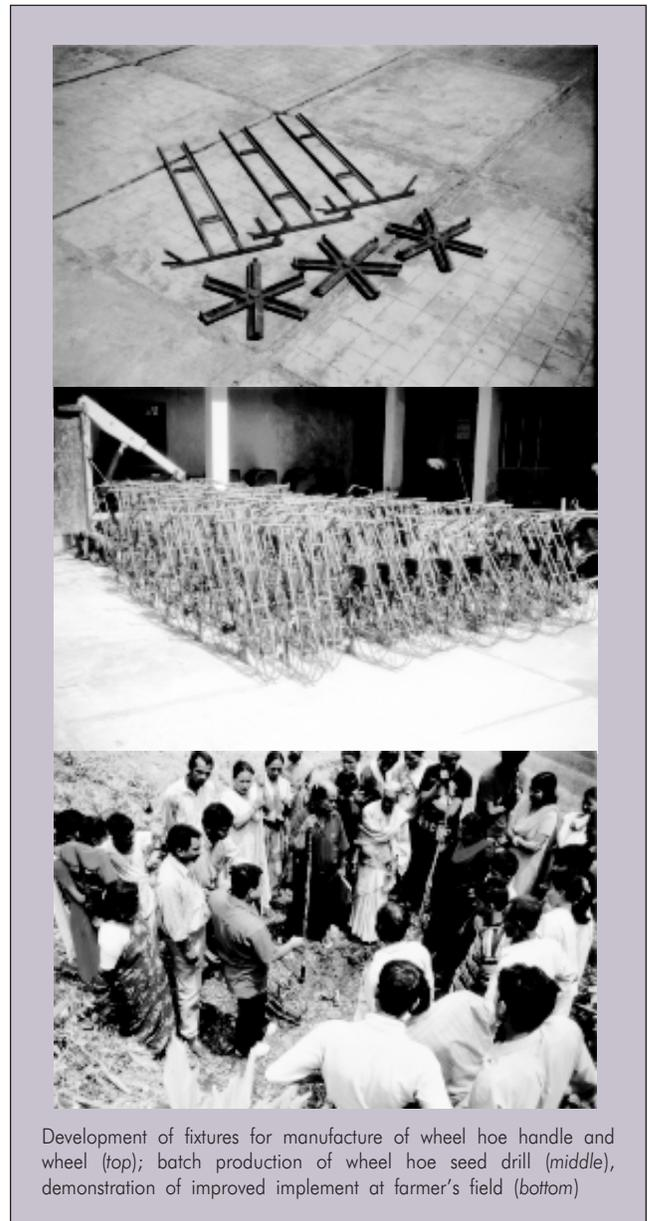
Development of fixtures for manufacture of wheel hoe handle and wheel (top); batch production of wheel hoe seed drill (middle), demonstration of improved implement at farmer's field (bottom)
