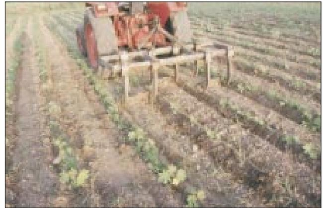
A tractor drawn 4-row weeder was developed. It can cover an area of 1.1 ha/hr.
