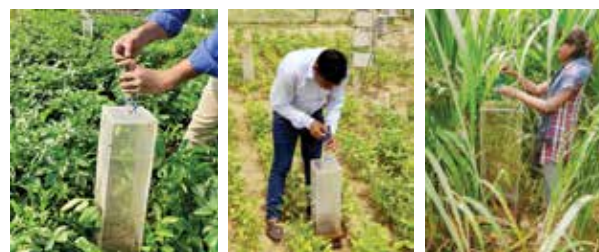
Sampling of GHG emission using close chamber technique in different crops
