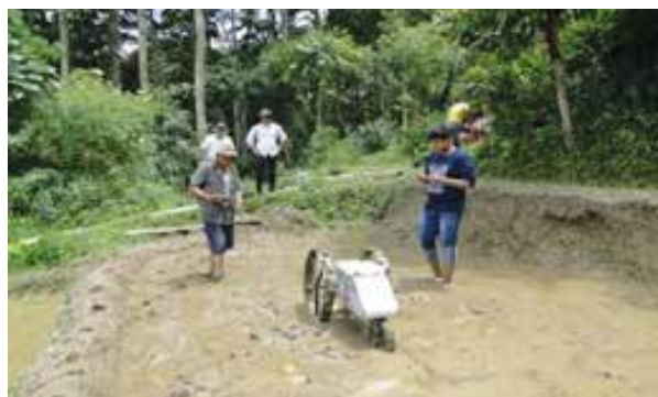
Remote controlled sensor based direct rice seeder
